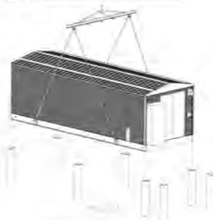
Figure 3 - Lifting onto Pile Caps
