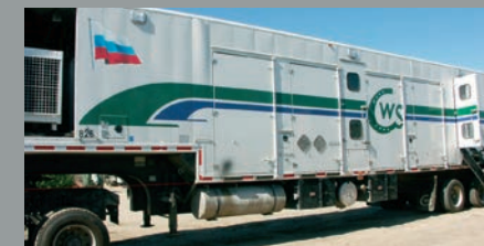
Calfrac Hydraulic Fracturing Trailer
